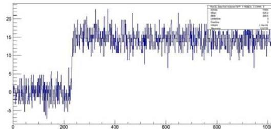
Figure 2: FEBEX signal trace with amplitude of 2 mV.
