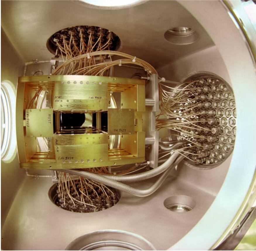
Detector for the measurement of the elements 107 and 112 discovered at GSI's SHIP experiment.
