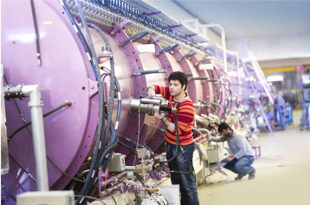
The GSI linear accelerator UNILAC was used to accelerate the ions in the production of elements 107 to 112. They are collided onto a material sample and form a new element by nuclear fusion
