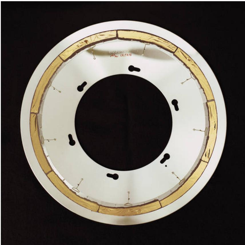
By colliding the ions brought to speed in the accelerator onto a target wheel, a new element can be produced by fusion of the atomic nuclei of both element types. The wheel in the picture is equipped with thin gold foil. When bombarded with ions, atoms of a new element can be formed. Due to the high impact velocity, they leave the foil and can be identified in a separate detector (see below).
