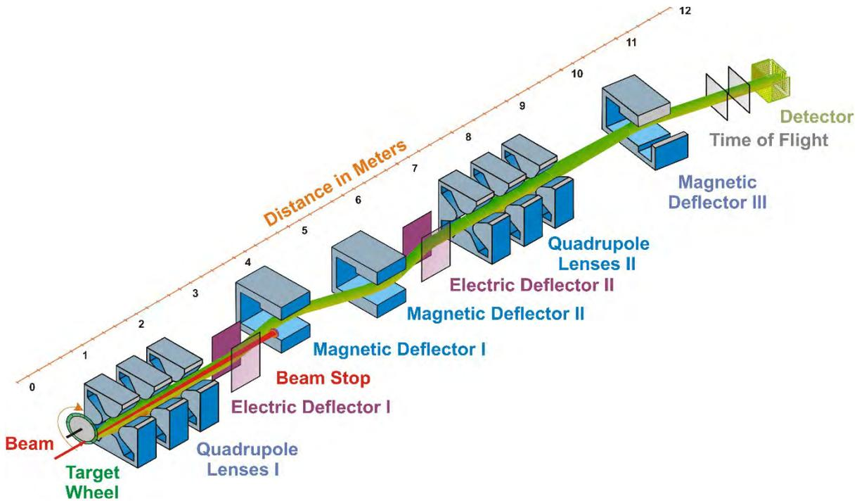
*Fig. 1:* The ion optical scheme of the velocity filter SHELs
